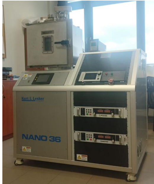
Figure 3.2. Thin Film Deposition System - NANO 36™ (Kurt J. Lesker Company) for producing low-dimensional structures.
