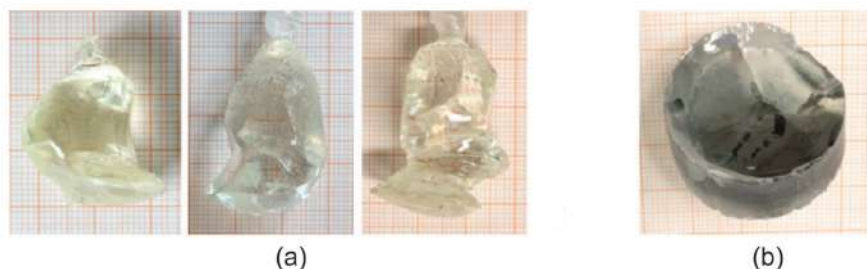
Fig. 4.9. a) Bulk \text{MgGa}_2\text{O}_4 single crystals obtained through the Czochralski method [153]; b) crystals obtained using the Kyropoulos-like method [100].
