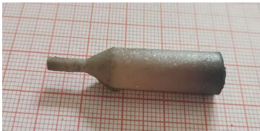
Fig. 3.4. An inorganic crystal of (Zn,Be)Se grown using the vertical Bridgeman method.
