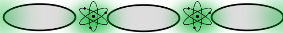
Fig.7 Sketch of geometry favourable to achieve the conditions of strong coupling, as discussed in the article [H6]. The field enhancement is strong in the gaps between the nanoparticles. The elongated shape of the nanoparticles is responsible for the strong confinement of the field at the prolate endings. Multiple atomic systems can be used to coherently enhance their interaction with the field.
